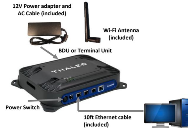
1. Open outer carton, remove BDU, AC adapter, AC Power and Ethernet Cables (or Wi-Fi antenna).
