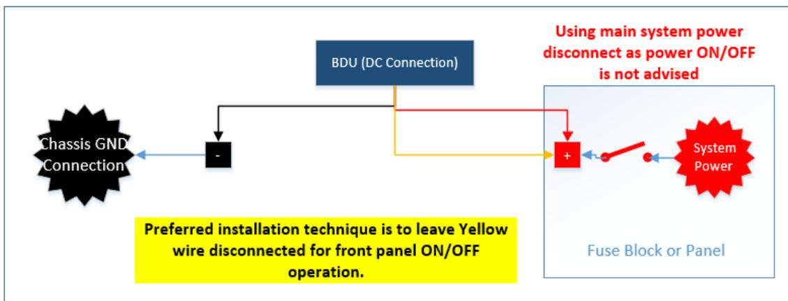
Figure 2-10: 24V DC Power Connection
