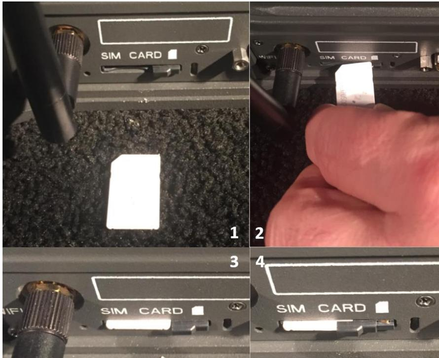
*Figure 2-7: Installing SIM Card and Engaging The Lock*
