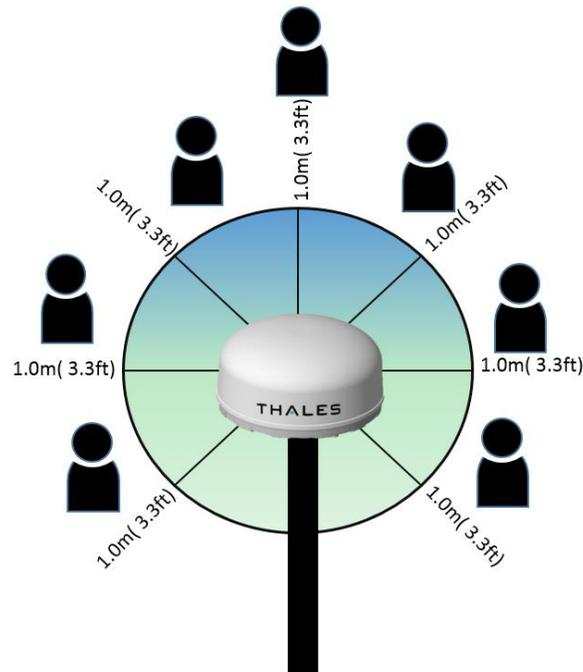
*Figure 1-1: MINIMUM Safe Distance From Antenna*
