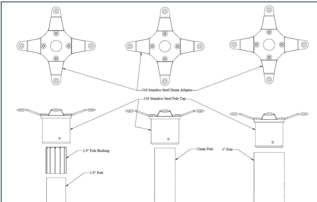
*Figure 2-5: Thales Antenna Mounting Bracket (Shown With Poles, Not Included)*
