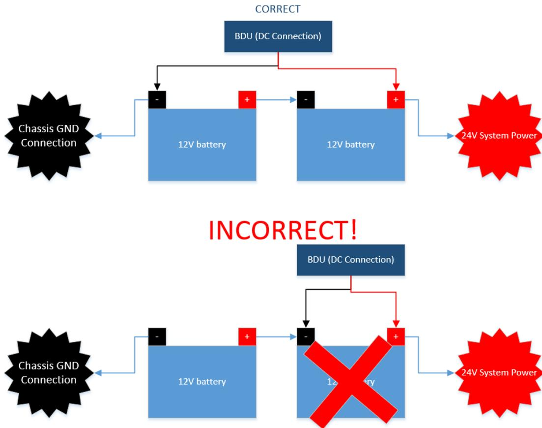
Figure 2-11: 24V DC Power Connection
