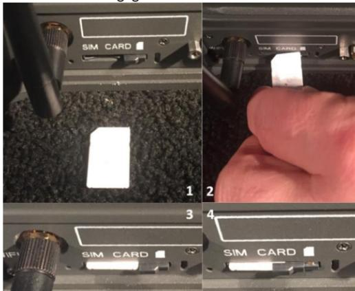
*Installing SIM card and engaging the lock*
