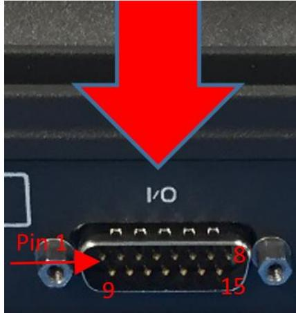
Figure 3-1 GPIO Connector Pin Detail
