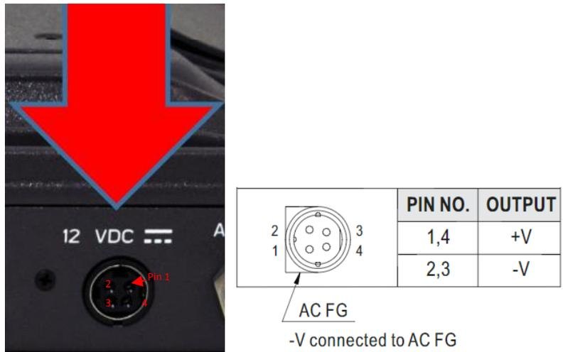
*Figure 3-2 12V Input and Mating Connector Detail*
