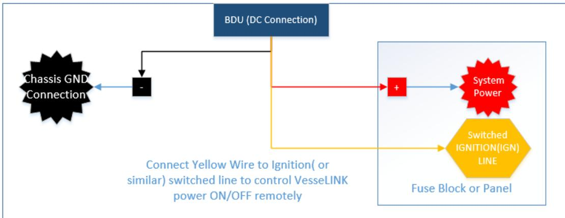
Connecting Yellow Wire directly to system power will disable VesseLINK power off capability.
