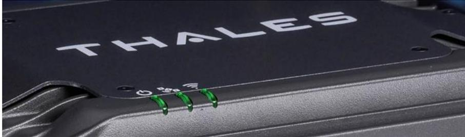
Figure 2-12: System Status Indicators (Top View of BDU)
