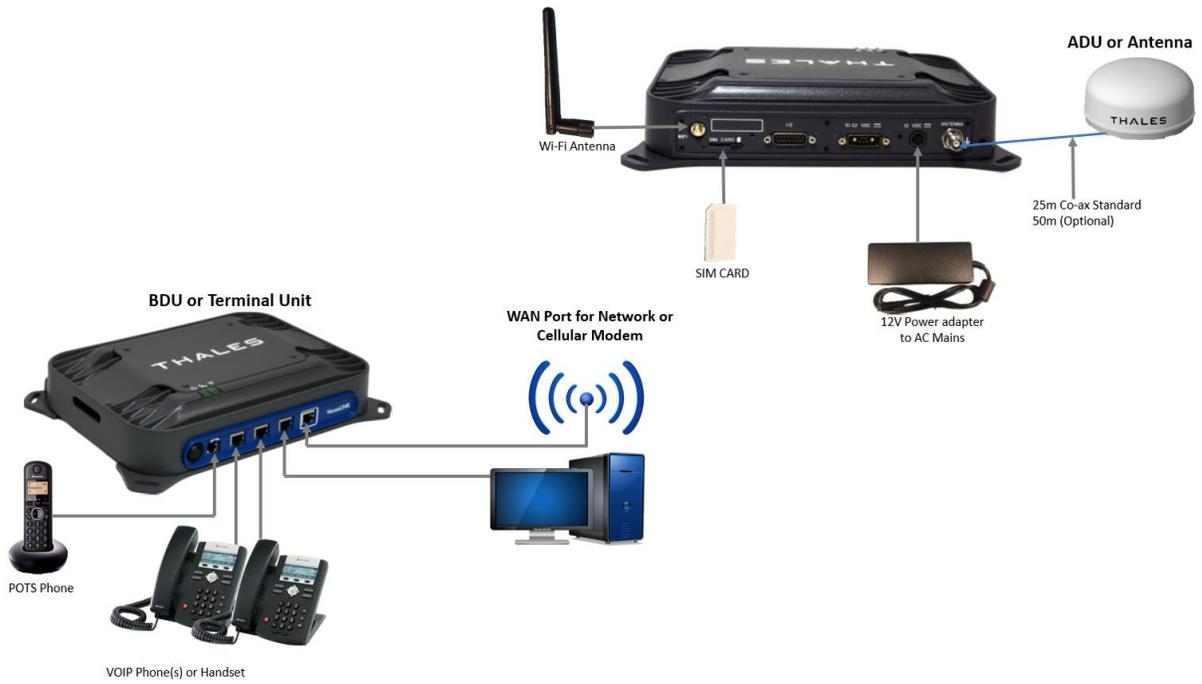
*Figure 1-2: VesseLINK System with Accessories*
