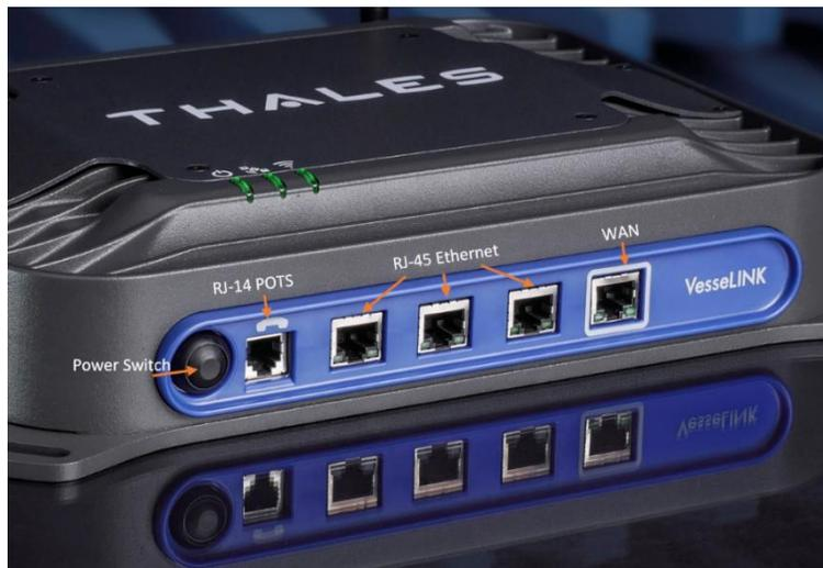
*Figure 1-4: BDU Front Panel Detail*
