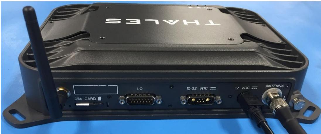
*Figure 2-8: Wi-Fi Antenna, SIM Card, AC/DC Power Adapter and Antenna Cable Installed*
