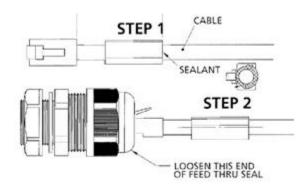
Figure 4-8 - Installing Ethernet Cable through fitting
