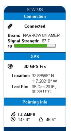
The status bar is included on the home page and other pages that do not have a navigation bar. It includes a field with the elevation angle and compass direction towards the visible satellite(s).
