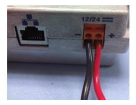
Figure 4-7 - Connecting power leads
