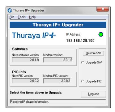
The 'New software version' indicates the software you are going to upgrade your Thuraya IP+. The 'Modem software version' indicates the software version currently loaded on your Thuraya IP+.
