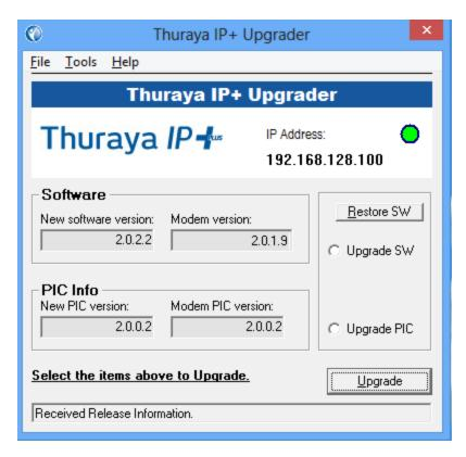
The 'New software version' indicates the software you are going to upgrade your Thuraya IP+. The 'Modem software version' indicates the software version currently loaded on your Thuraya IP+.
