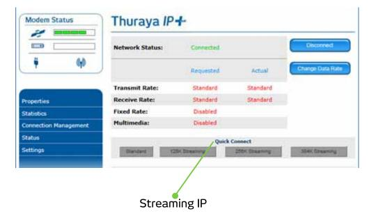
1 - Connecting to Streaming IP: On the wMMI, press the desired symmetric Streaming IP connection speed. The network status changes to "Acquiring" and then to "Connected".
