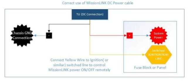
Figure 2-7 10V - 32V DC Power Connection
