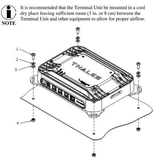
Figure 2-3 Terminal Unit Mounting Detail
