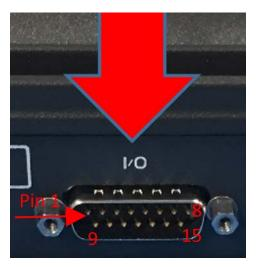
Figure 4-1 GPIO Connector Pin Detail
