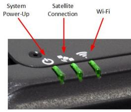
Figure 1-3 Terminal Unit (TU) LEDs
