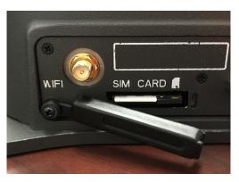
Figure 2-4 SIM Card with Cover Opened
