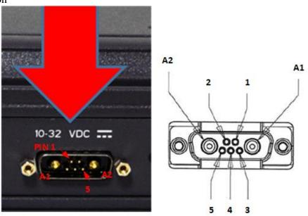
Figure 4-3 10-32 VDC and Mating Connector Detail
