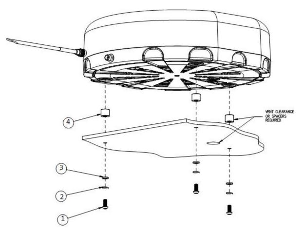
Figure 2-2 Hard Mount Antenna
