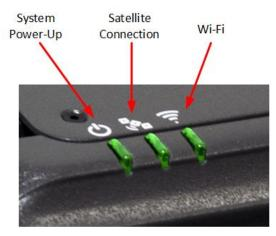
Figure 2-9 Terminal Unit (TU) LEDs
