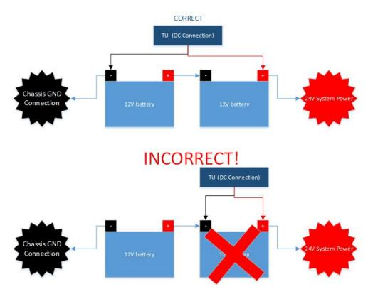
Figure 2-8: 24V DC Power Connection
