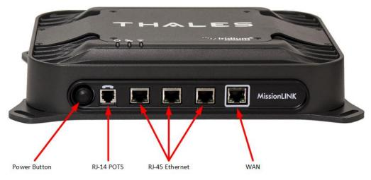
Figure 1-4 Terminal Unit (TU) Front Panel Detail
