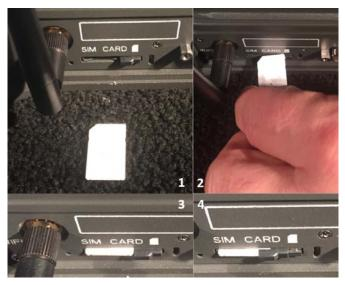
Figure 2-5 Installing SIM Card and Engaging the Lock
