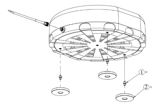
Figure 2-1 Magnetic Mount Antenna
