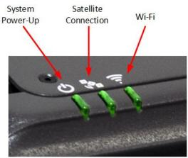
Figure 2-5 Terminal Unit (TU) LEDs
