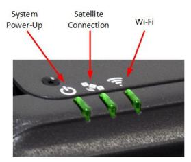
Figure 3-6 System, Satellite and Wi-Fi Status LED's
