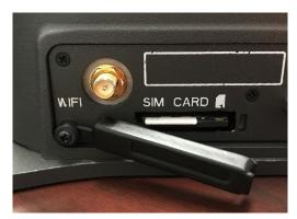
Figure 3-3 SIM Card with Cover Opened
