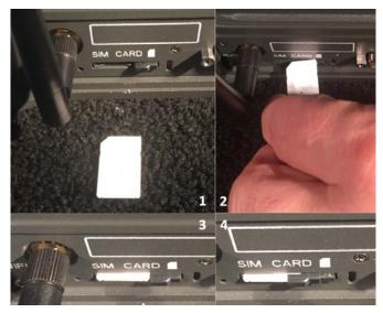
Figure 3-4 Installing SIM Card and Engaging the Lock
