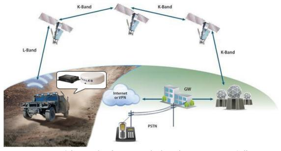
Figure 1-2 Typical Iridium Network Flow of a Voice or Data Call.
