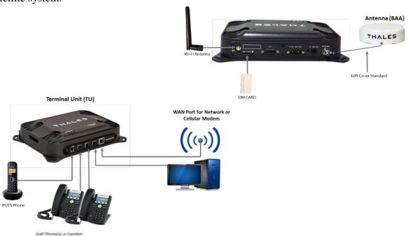
Figure 2-3 MissionLINK™ System with Connected Hardware
