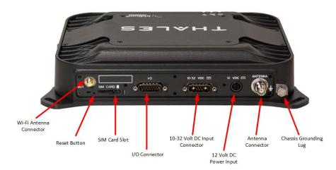
Figure 2-7 Terminal Unit (TU) Back Panel Detail
