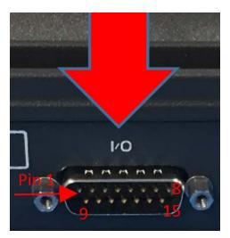
Figure 7-2 GPIO Connector Pin Detail
