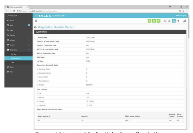
Figure 4-41 Diagnostics → Satellite Modem Screen (Sheet 1 of 2)
