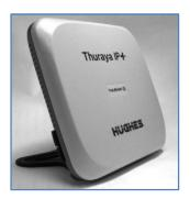
Access Point in the Thuraya IP+ uses a separate subnet and DHCP server than the wired Ethernet port. An internal router allows IP traffic to flow seamlessly between the two subnets and out over the satellite link.
