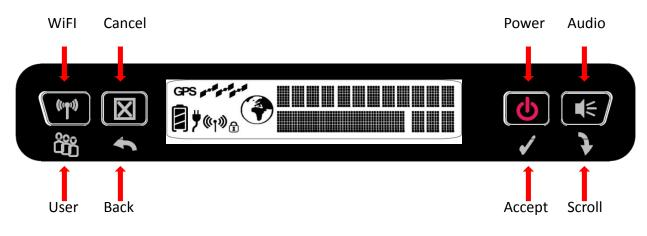
The top line gives the compass bearing and elevation angle of the closest satellite.
