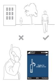
Note: Before you make a call, your phone needs a GPS fix so it can be located by the satellite. This happens automatically, but if a new GPS fix is needed, the council icon will be displayed. Place the phone in the open with a clear view of the sky until the council icon disappears.
