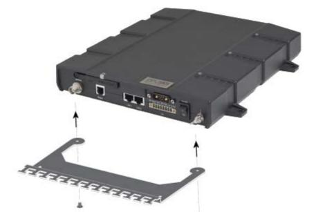
2. Fasten the Basic cable support to the terminal using two M4 x 6 mm countersunk screws.
