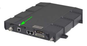
Insert the SIM card into the SIM slot. Place the card with the chip side facing up as shown.
