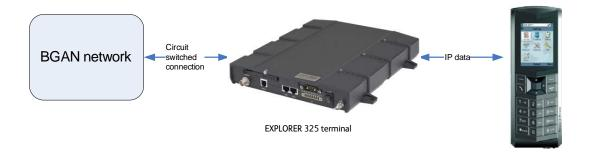
When connected to the terminal the IP Handset provides a dedicated BGAN menu with a subset of the terminal configuration options.
