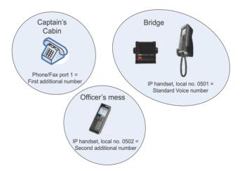
Note that you can also assign the call type numbers directly (in the example above, the Standard Voice number is assigned to IP handset number 0501). If you do so, be aware that only the assigned handset can receive a call to this number. The handset connected to Phone port 1 and the IP handset no. 0501 are each assigned an additional number. For details on additional numbers, see Additional numbers for Multi-voice on page 61.
