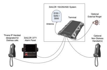
**To make a Distress call**: Push and hold the red button on the alarm panel for 5 seconds. When the Distress IP Handset rings, pick up the phone. You are now put through to the nearest rescue centre. Follow the procedure for Voice Distress calls.
