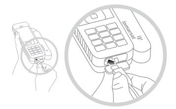
Connect the charger to a power source and the micro USB connector to the port at the base of the phone, under the USB/audio protective cover.
