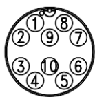
Figure 36: AUX connector (pin out)
