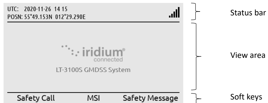
Figure 46: LT-3110S Control Unit (display sections)
