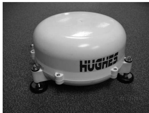
Figure 6-2 C11 antenna unit
