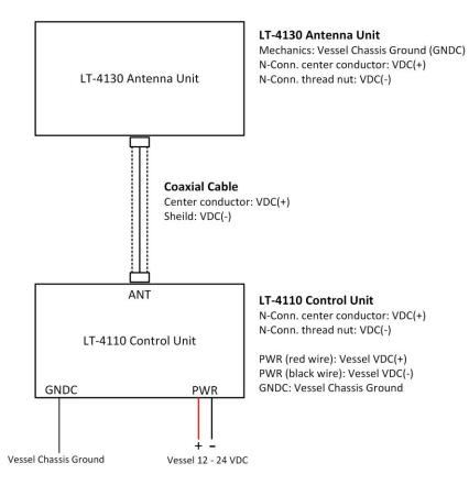
Figure 32: Definitions of VDC (+), VDC (-), and GNDC
