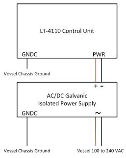
Figure 33: AC/DC Galvanic Isolated Power Supply
