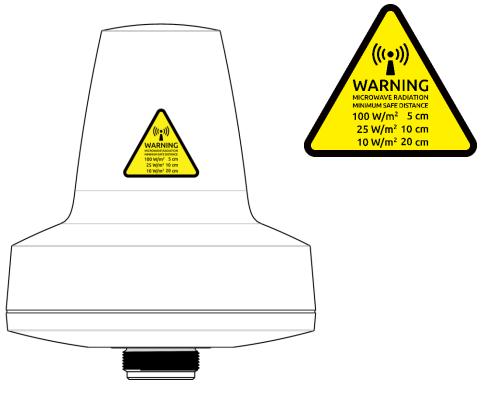
Figure 12: LT-4130 Antenna Unit (incl. warning label)
