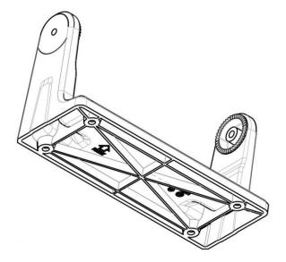
Figure 4: Bracket Mount, Control Unit.
