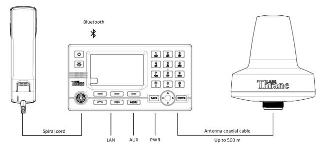
Figure 1: LT-4100 system - basic components and interfaces.
