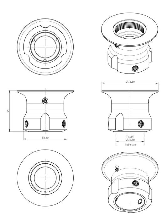
Figure 153: Outline Drawing: Pole Mount (1.5" pipe), Antenna Unit
