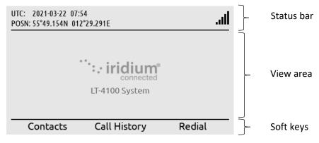
Figure 36: LT-4110 Control Unit - UI display sections
