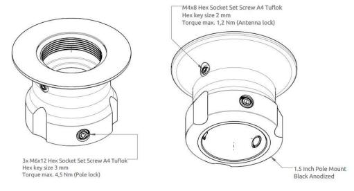
Figure 19: Pole Mount (1.5" pipe), Antenna Unit.
