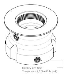
Figure 22: Pole Mount (2.0" pipe), Antenna Unit.
