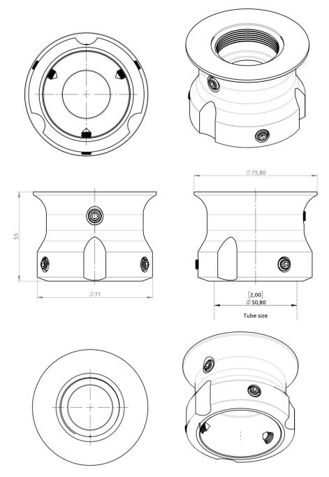
Figure 154: Outline Drawing: Pole Mount (2.0" pipe), Antenna Unit
