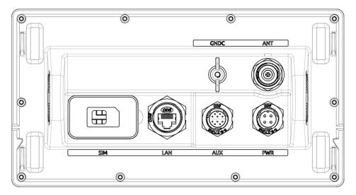
Figure 24: LT-4110 Control Unit (back view)
