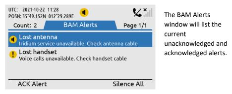
Figure 101: LT-4110 Control Unit (BAM Alert list)
