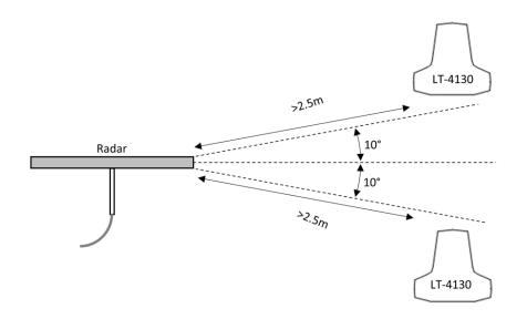
Figure 13: LT-4130 Antenna Unit – Avoid Radar Beam
