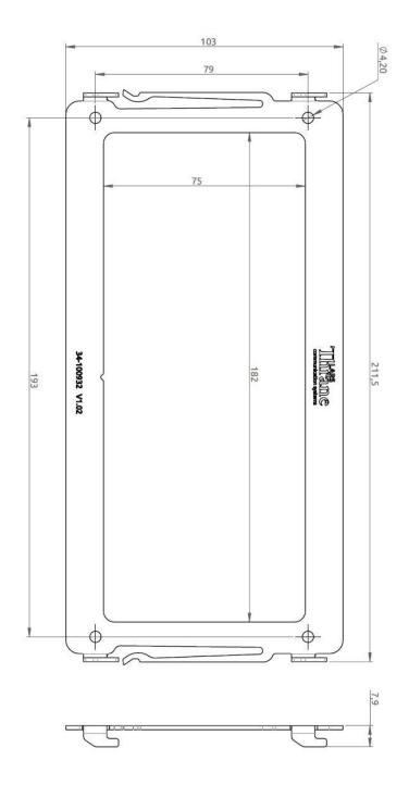
Figure 151: Outline Drawing: Flush Mount, Control Unit
