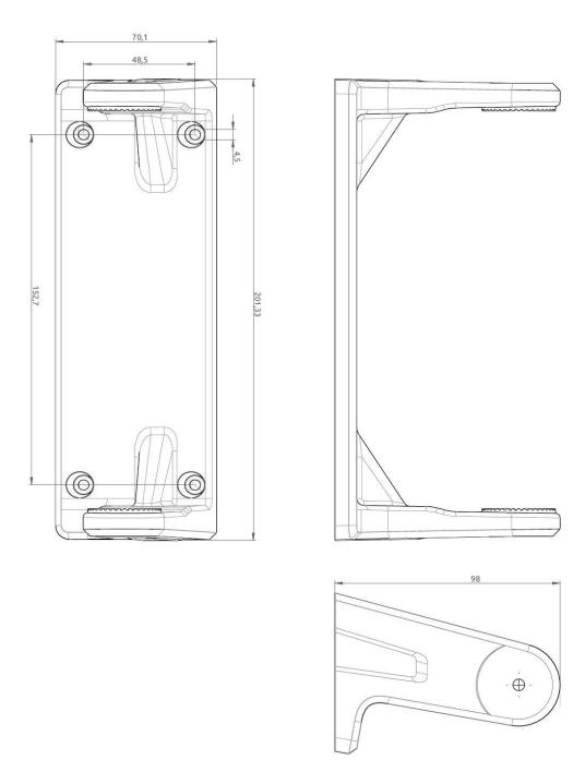
Figure 150: Outline Drawing: Bracket Mount, Control Unit
