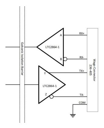
Figure 28: RS-422 Circuit Diagram for the LT-4110 CU
