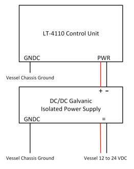
Figure 34: DC/DC Galvanic Isolated Power Supply
