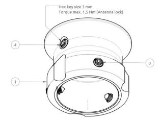
Figure 23: Pole Mount (2.0" pipe), Antenna Unit.
