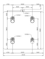
The mounting location hole (unit: mm)
