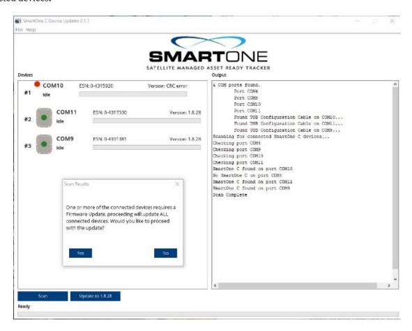
5. To initiate the firmware updating process, press the "Update to x.x.xx" ("x.x.xx" will be the current version number) button located at the bottom left of the main dialog screen.
