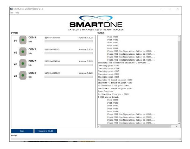
**NOTE:** If the SmartOne C Firmware Device Updater program fails to locate a connected S1C device, you may have to disconnect and reconnect the S1C device and/or its USB Configuration cable. Then select the Scan button to re-scan connected S1C devices.
